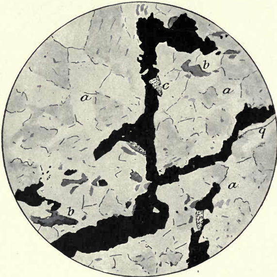
Replacement-Vein in Syenite Rock. War Eagle mine, Rossland, British Columbia. a , Granular aggregate of orthoclase with very little sericite; black, secondary pyrrhotite; b , secondary biotite; q , secondary quartz; c , chlorite. Magnified 60 diameters.
